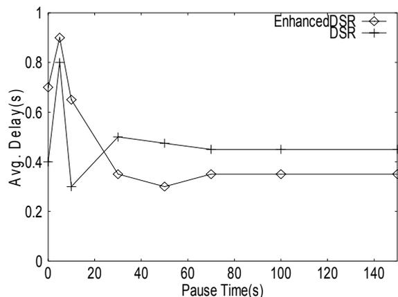
Fig.6: Delay Vs Mobility for Model2
