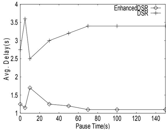
Fig.4: Delay Vs Mobility for Model1
